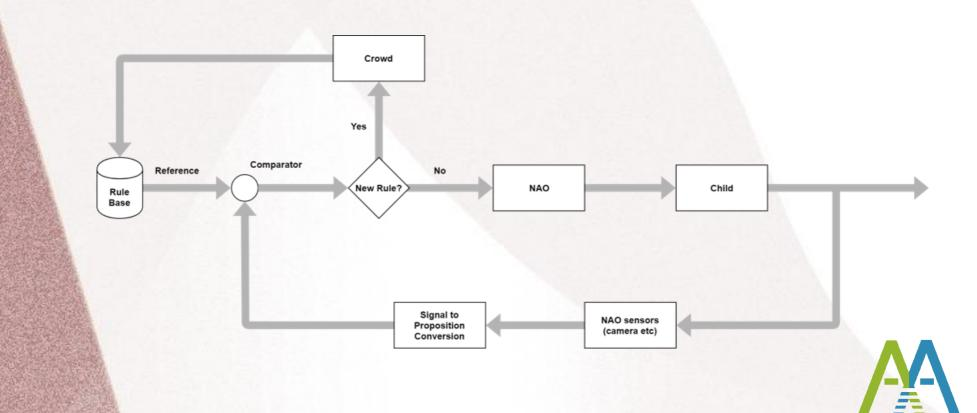
b. The Rule Base calculates a Reference proposition p<sub>R</sub> as an input to a Comparator.
