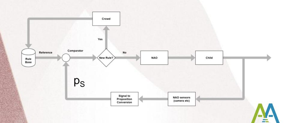
d. The propositions p<sub>R</sub> and p<sub>S</sub> are compared toward driving a Linguistic Controller (in the NAO robot) toward bringing the Child to the desired Reference.
