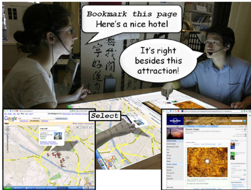
Figure 2.4: IMT using voice and multitouch interaction based in the DiamondTouch multitouch surface by MERL.
