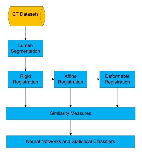
Figure 7.2.: Pipeline of the CAD system for EVAR evolution prediction from image data.
