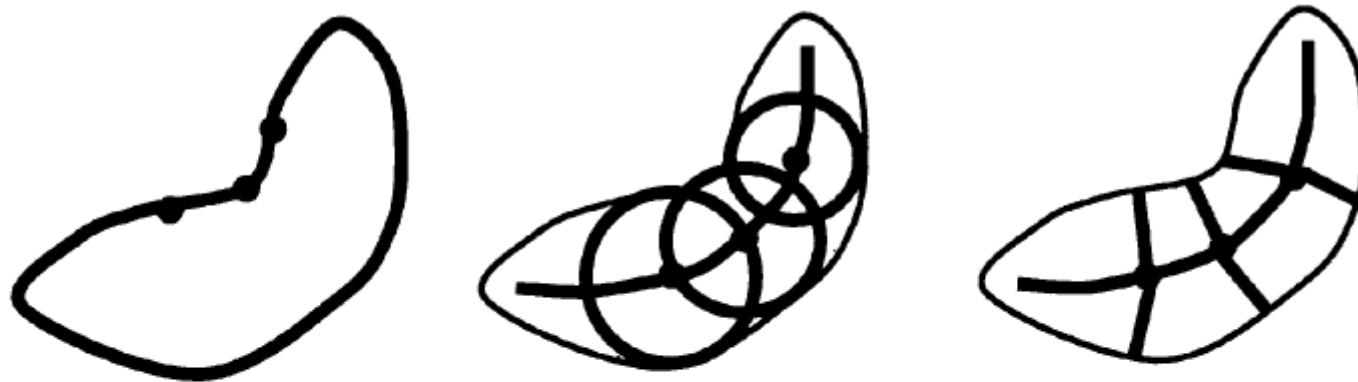
Fig. 1. 2-D figure shown in terms of its boundary, then in terms of bitangent circles wholly interior to the figure, and finally, in terms of medial atoms (see also Fig. 5 for the 3-D case). Individual positions, circles, and medial atoms are shown at sample positions, but in each case, the locus is continuous. The part of this figure that forms the representation is shown in each case with bolder lines.
