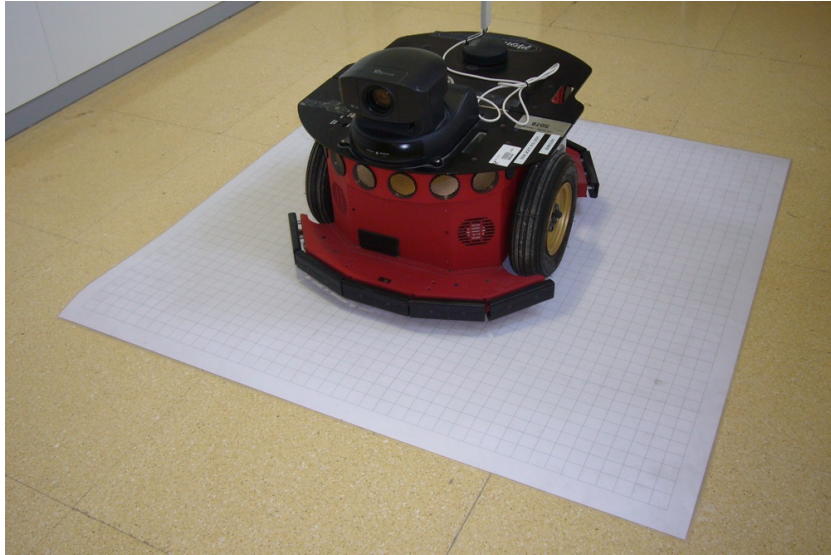
Figure C.12: Pioneer 2 DXE on the graduated sheet used to measure position recognition area.
