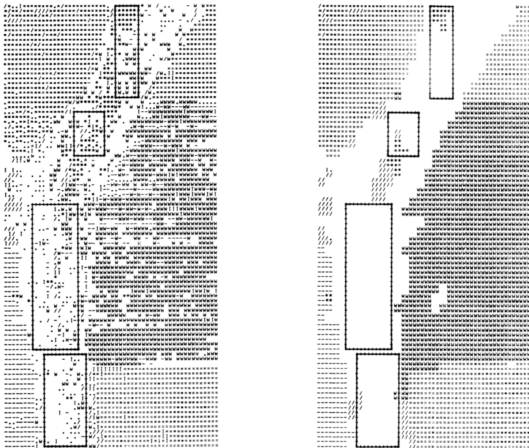
Fig. 3. Logogrammatic classification maps produced by no-memory classifier (left) and sample classifier (right).
