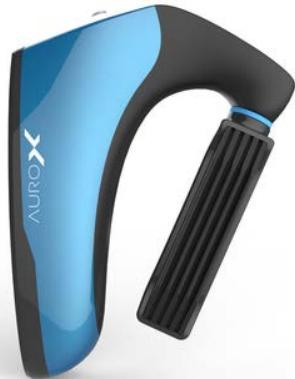
Aurox is a portable device that cools inflamed skin at the entry of the ear canal; directly targeting the areas of pain for those suffering from outer ear infections (otitis externa). This handy device, which utilizes thermo-electric cooling, is able to control optimum temperatures in order to relieve patients' discomfort.
