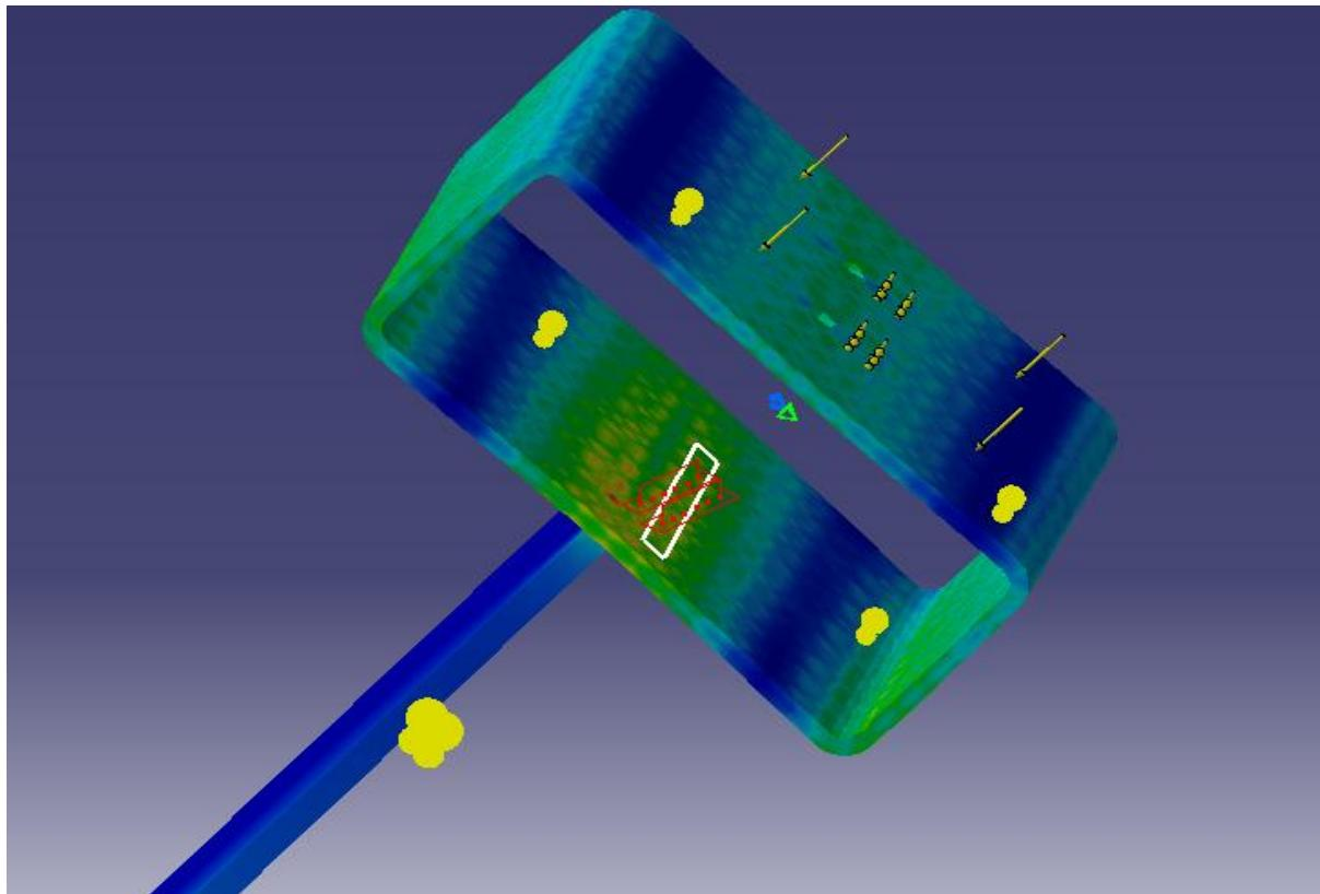
**Simulate the mechanical behavior of a beam, which is supporting a facade**
