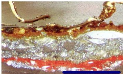
**fig 1.** Paint stratigraphy: from inner to outer: gypsum base, clay-rich primer, gypsum layer with dissolution pores and re-crystallized gypsum (arrow-like crystals), clay-rich layer and tin coat exhibiting bowl-like shapes and detachments. Transmitted light and crossed nicols. Bar = 0.5mm.
