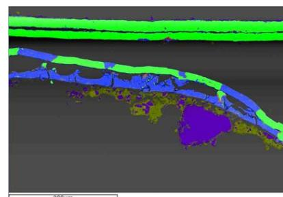
fig. 5. False color map of a paint stratigraphy showing the fresh (light grey/green) and oxidized (dark grey/blue) tin layers.
