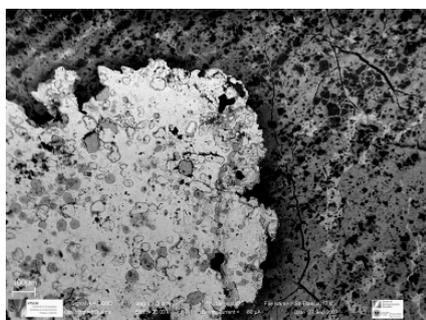
fig. 2. Contact between the light grey less corroded and the intensely altered dark grey tin layers.
