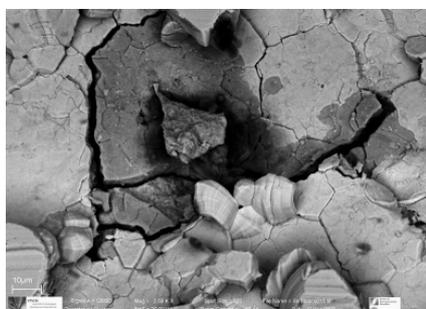
fig. 3. Tin whiskers extruding from polygonal cracks.
