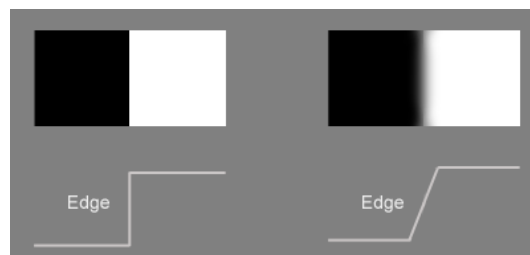
Figure A.9: (Left) Two surfaces ideally perfectly in focus, (Right) Soft boundary transition between two unfocused surfaces.
