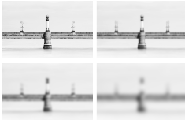
Figure 2.3: Smoothed versions of original image for Scale-space representation at t=1, t=4, t=8 and t=16
