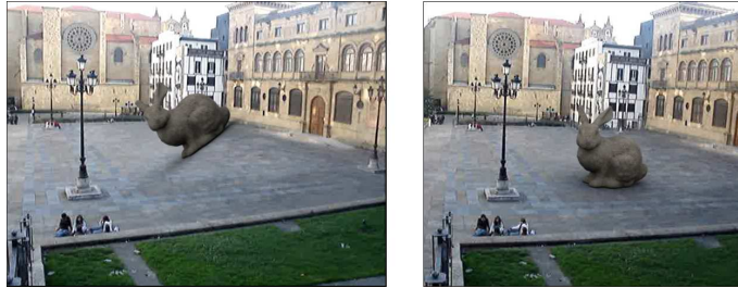
Figure 5.3: (left) Wrong camera pose estimation, (right) Correct camera pose estimation, the virtual object appears correctly aligned with real world.
