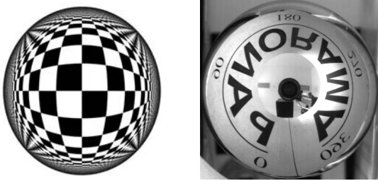
Fig. 1: (a) A simulated checkerboard wall viewed by camera looking at spherical mirror (b) Image captured using spherical mirror. The camera is the black object at the center. Image courtesy of http://cmp.felk.cvut.cz/demos/Omnivis/index.html
