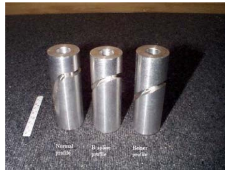
Figure 1 Three cylindrical cams machined with CNC programs generated by CYLCAM
