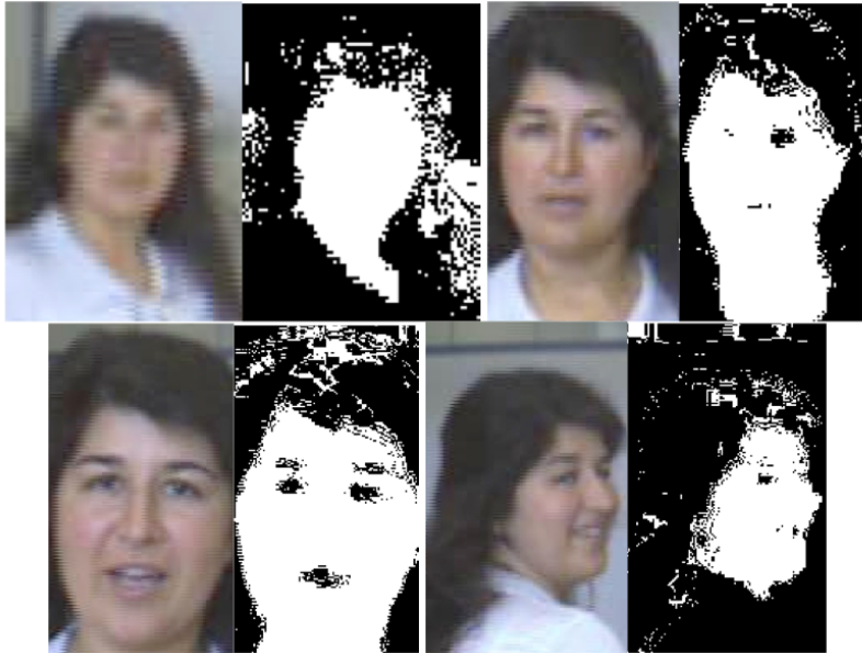
Figure 13.5: Results of pixel classification on images selected by the signature algorithm.
