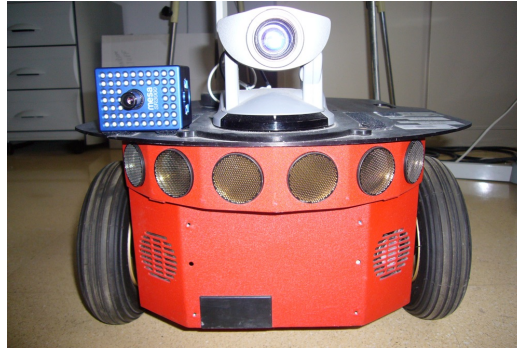
Figure C.14: 3D camera mounted on the Pioneer robot.
