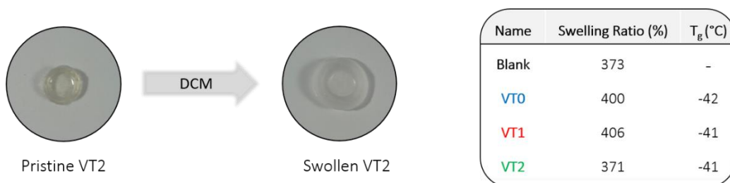
Figure 2.11: Picture representing pristine VT2 (left) and the swollen in CH 2 Cl 2 counterpart (left panel) and swelling ratio and T g data for each formulation of vitrimer VT0, VT1 and VT2 and control crosslinked network blank.
