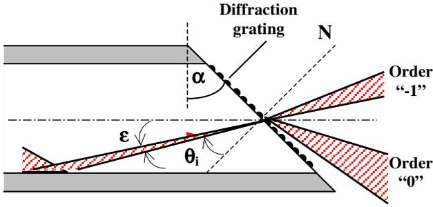
**Figure 2.** Diffraction caused by a diffraction grating located in the extremity of a tilted fibre. Order (-1) and order 0 mean diffraction orders -1 and 0.
