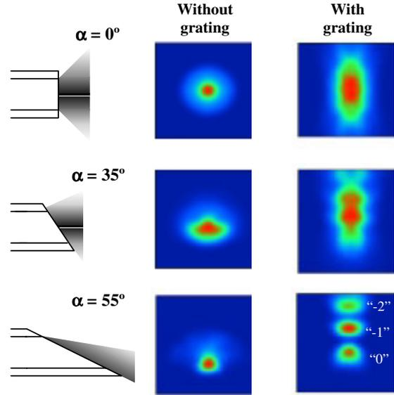
**Figure 3.** Intensity patterns of the light irradiated by an end face fibre tilted for  $\lambda = 660 \text{ nm}$ .
