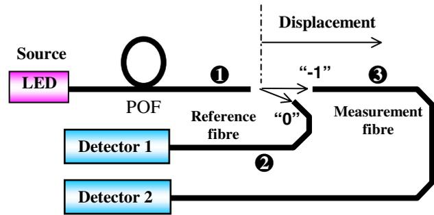
**Figure 5.** Scheme of the proposed displacement sensor. This consists of an emitting fibre, with its diffraction grating, and two receiving fibres: one for the order 0 (fibre 2), which serves as a reference, and the other for the order  $-1$  (fibre 3), which measures the displacement.
