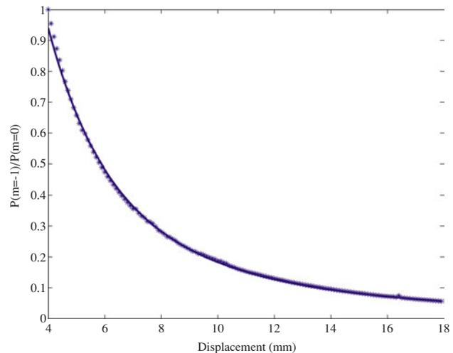
**Figure 6.** Relative power of the order  $m = -1$  with respect to the order  $m = 0$  against displacement for a wavelength of  $660 \text{ nm}$ . The experimental data are plotted with asterisks and the best fitting curve with a continuous line.
