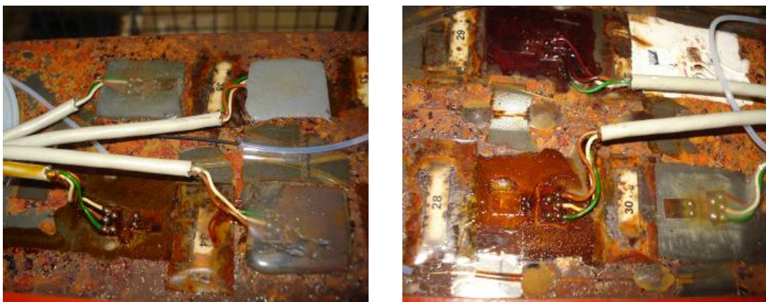
Figure 5. State of the gauges and FBGs after aging on climate chamber.
