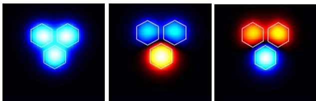
Fig. 2. Simulated mode profiles of the three polarization degenerate supermodes supported by the three-core MCF shown in Fig. 1.
