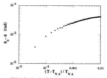
FIG. 8. Log-log plot of the tilt angle relative to its value at  $T_{NA}$  vs the reduced temperature above the  $N^*$ -Sm-A transition.
