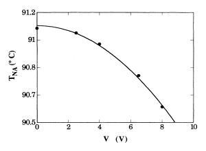
FIG. 5. Voltage dependence of the effective temperature of the  $N^*$ -Sm-A phase transition. The continuous line is the best fit to a quadratic law,  $T_{NA}(V) - T_{NA}(0) \propto V^2$ .
