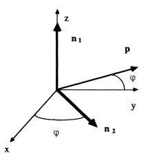
FIG. 1. Schematic description of the orientation of a chiral molecule.  $\mathbf{n}_1$  is the usual nematic director and  $\mathbf{n}_2$  is a second director orthogonal to  $\mathbf{n}_1$ , which accounts for the orientation of other transverse molecular parts. The molecule is supposed to have a lateral dipole moment given by  $\mathbf{d} = \mu \mathbf{n}_1 \times \mathbf{n}_2$ .
