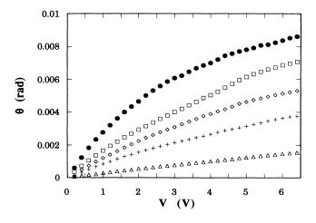
FIG. 2. Induced tilt angle as a function of the applied voltage in the Sm-A phase. The five curves correspond to the following temperatures: T=62.5, 63.0, 63.5, 64.0, and 67.0°C. A strong nonlinear behavior near the Sm-A-Sm-C\* transition can be observed.
