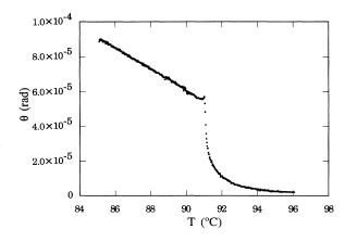
FIG. 7. Temperature dependence of the tilt angle induced by a sine-wave voltage of 2.5 V and 1 kHz around the  $N^*$ -Sm-A phase transition.
