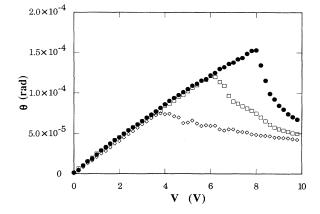
FIG. 4. Induced tilt angle as a function of the applied voltage around the  $N^*$ -Sm-A transition. The decreasing behavior above a certain threshold is due to the electric field dependence of  $T_{NA}$ . The circle, square, and tilted square symbols represent T=90.6, 90.8, and 91.0 °C, respectively.
