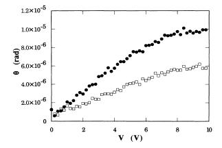
FIG. 6. Induced tilt angle as a function of the applied voltage in the  $N^*$  phase. The circle and square symbols refer to T=94.0 and 96.0 °C, respectively.
