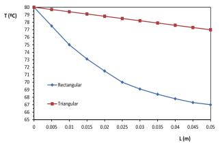
**Figure 9:** Surface temperature distribution for rectangular and triangular fin respectively.
