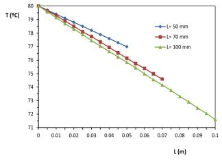
**Figure 8:** Surface temperature of the fin for L = 50, 70 and 100 mm. respectively.
