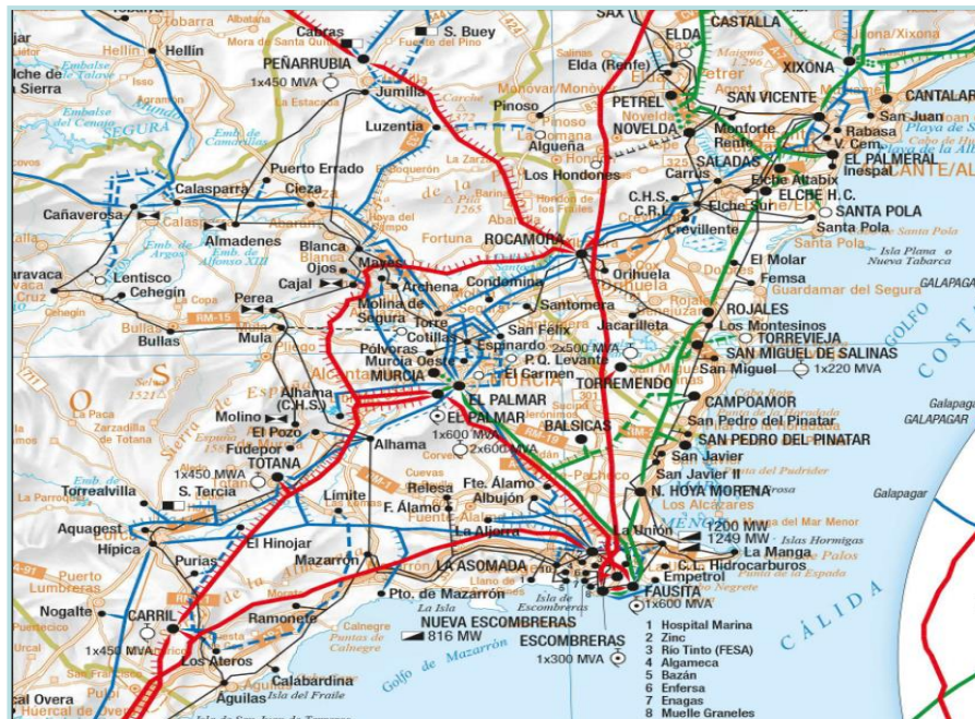
Figure 10. 220kV Murcia interconnector affected by the N-2 outage
