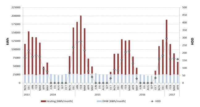
Fig. 9. Calculated monthly energy consumption used in the building for heating and DHW, and HDD during the four heating seasons studied (November 2013-April, 2017)
