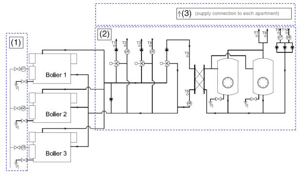
Fig. 4. Energy system for DHW and heating
