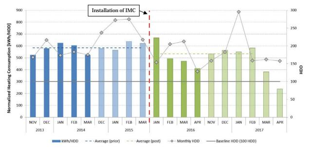
Fig. 10. Monthly average amount of weather-normalized heat used in the building and HDD during the four heating seasons studied (months when HDD>100; energy data source: [A] in Table 2)
