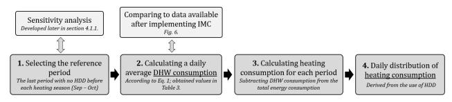
Fig. 8. Workflow of the method followed for disaggregating values of DHW and Heating consumption
