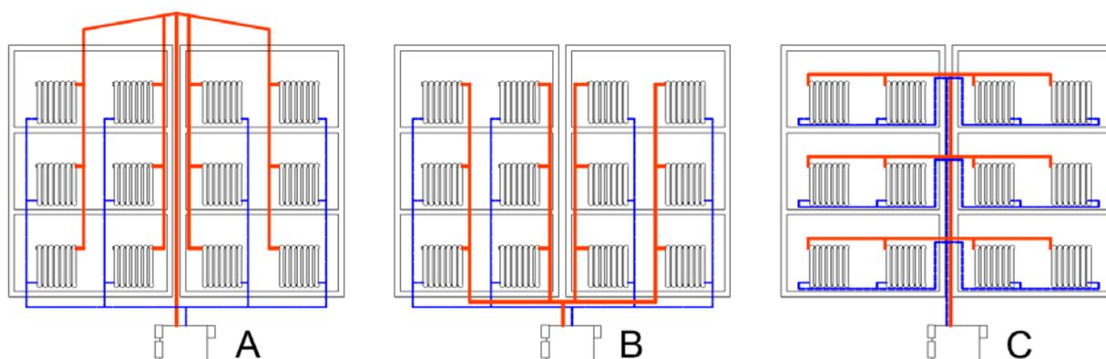
Fig. 1. Different heating system configurations (A: thermosiphon heat pipes; B: vertical pipes with forced circulation; C: ring circuit network)
