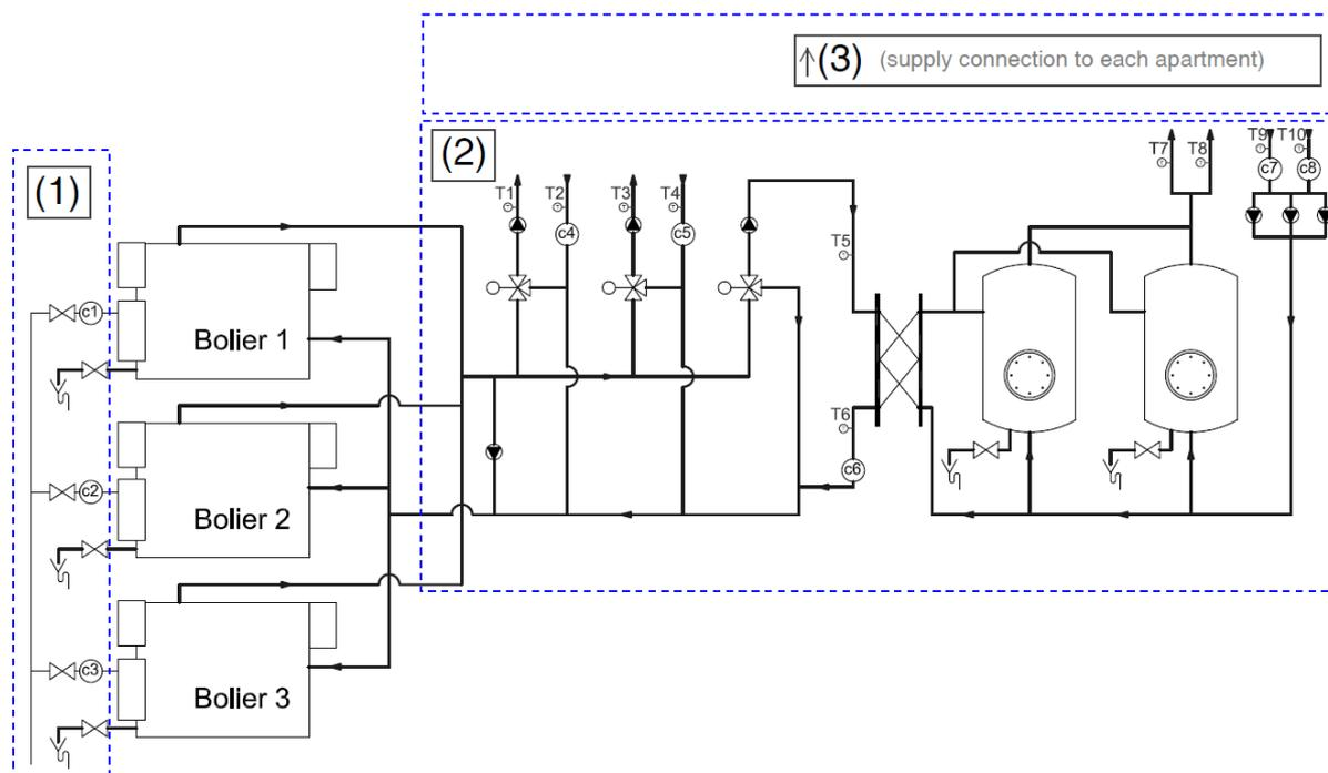
Fig. 4. Energy system for DHW and heating
