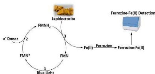
Figure 1. Proposed catalytic cycle for the reduction of Lepidocrocite to Fe(II) mediated by FMN and Ferrozine.
