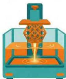
Figure 1. Representation of Vat Photopolymerization
