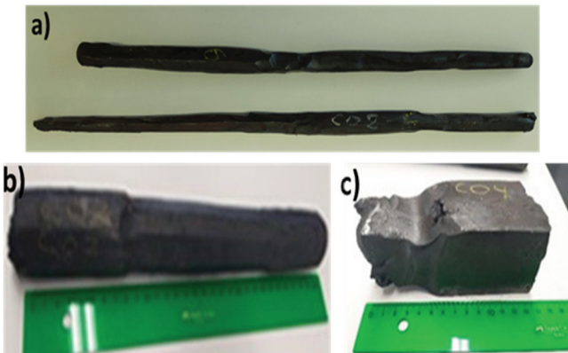
Figure 6. Forged ingots. (a) 1 Kg of austenitic and duplex low-density steels, (b) 5 Kg duplex low-density steel, and (c) 5 Kg austenitic low-density steel burst.
