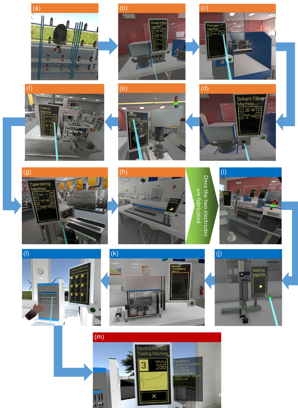
Figure 4. Various process steps that are possible to undertake in our BMM. The orange labels correspond to electrode manufacturing processes, and the blue labels correspond to the final cell manufacturing processes. The result shows the gravimetric cell energy density of the fabricated cell, along with the typical GCPL curve associated with the chosen chemistry combination of the electrodes, and a feedback on the parameters chosen during the fabrication. Each machine requires an input object (product/material) to start the process. a) Chemistry selection; b) power filling; c) premixing; d) solvent filling; e) mixing; f) coating and drying; g) calendaring; h) electrode cutting; i) winding; j) welding; k) degassing + electrolyte filling; l) formation and testing; m) result.
