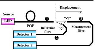
**Figure 5.** Scheme of the proposed displacement sensor. This consists of an emitting fibre, with its diffraction grating, and two receiving fibres: one for the order 0 (fibre 2), which serves as a reference, and the other for the order -1 (fibre 3), which measures the displacement.
