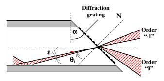
**Figure 2.** Diffraction caused by a diffraction grating located in the extremity of a tilted fibre. Order (-1) and order 0 mean diffraction orders -1 and 0.
