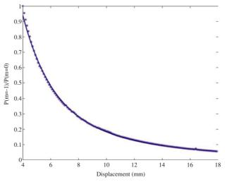
Figure 6. Relative power of the order m = -1 with respect to the order m = 0 against displacement for a wavelength of 660 nm. The experimental data are plotted with asterisks and the best fitting curve with a continuous line.
