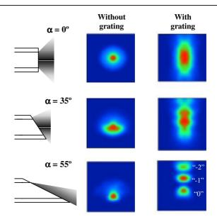
Figure 3. Intensity patterns of the light irradiated by an end face fibre tilted for  $\lambda = 660$  nm.
