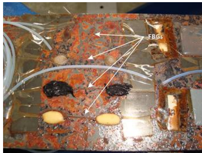
Figure 3. Photograph of four FBGs bonded with different adhesives to the F114 steel specimen after being aged for two months in a climate chamber.
