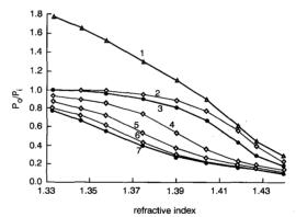
**Fig.4** Method to obtain a more linear curve by adding a concave one and a convex one 1) R = 8 + R = 4.25; 2) R = 9mm; 3) R = 8mm; 4) R = 6mm; 5) R = 5mm; 6) R = 4.5mm; 7) R = 4.25mm
