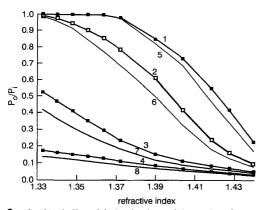
**Fig.6** Combined effect of the bend radius and the number of turns 1) 0.5 turns; R = 15mm; 2) 0.5 turns; R = 9mm; 3) 0.5 turns; R = 4mm; 4) 0.5 turns; R = 1.75mm; 5) 1.5 turns; R = 1.5 turns; R = 9mm; 7)1.5 turns; R = 4mm; 8) 1.5 turns; R = 1.75mm
