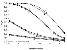
**Fig.7** Comparison between 10,000 rays  $(1^{\circ})$  and 2.56 million rays  $(2^{\circ})$ 1) R = 15mm  $(1^{\circ})$ ; 2) R = 15mm  $(2^{\circ})$ ; 3) R = 9mm  $(1^{\circ})$ ; 4) R = 9mm  $(2^{\circ})$ ; 5) R = 4mm  $(1^{\circ})$ ; 6) R = 4mm  $(2^{\circ})$ ; 7) R = 1.75mm  $(1^{\circ})$ ; 8) R = 1.75mm  $(2^{\circ})$
