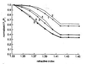
**Fig.9** Comparison between experimental and theoretical results 1) R = 12 mm; 2) experimental; 3) R = 7 mm; 4) experimental; 5) R = 4 mm; 6) experimental
